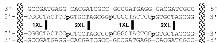
Scheme 4. Schematic representation of the procedure for the construction of the DNA nanostructures with cross-linked oligonucleotides by self-assembly of the DNA and subsequent DNA ligation. The bold bars represent cross-linkers.
